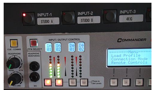
Signal strength indication (above). The system is fitted with a limiter which adjusts the volume and tone qualities and ensures consistent volume levels.
