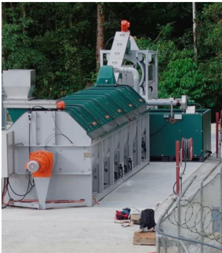
Figure 6 Vessel composting system (HotRot 1811 Composting Unit | Global Composting Solutions)
