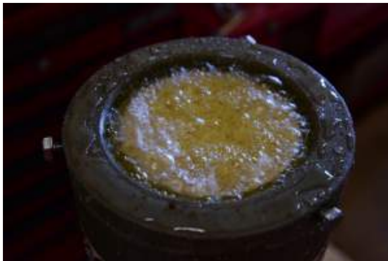
Figure 3. Module L1 from unit B at 40 kPa in a pinning repair tube showing the majority of fibres bubbling on the outside of the bundle.
